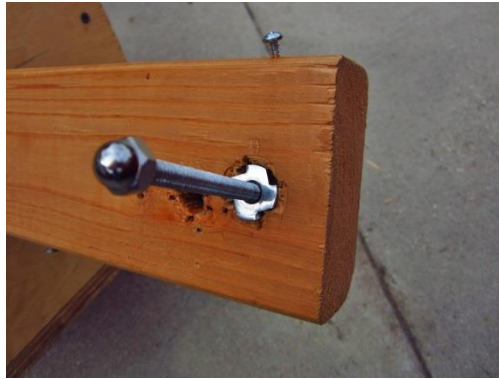
Figure 10: The screw supports the top lever through a loosely attached T nut.
