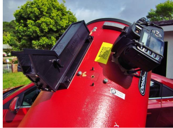
Figure 18: Rebel XT attached with rubber bands next to the Telrad.
