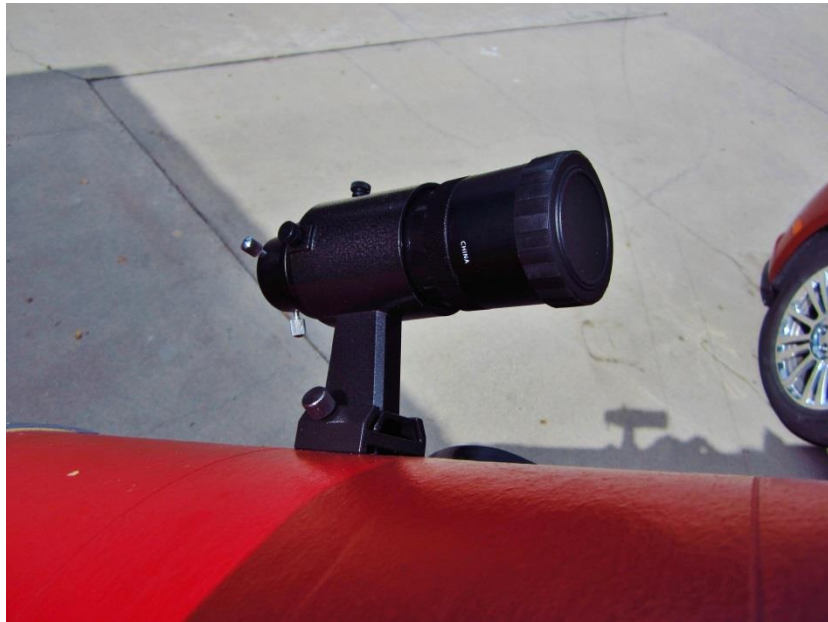
Figure 19: The guide scope mounted near the OTA center of mass.
