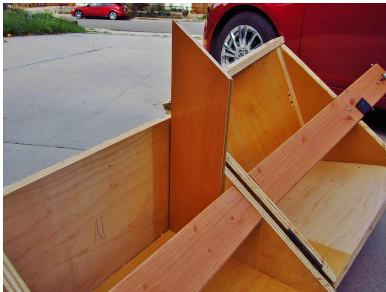
Figure 9: The alignment plank is pressed against the hinge board to help with polar alignment.
