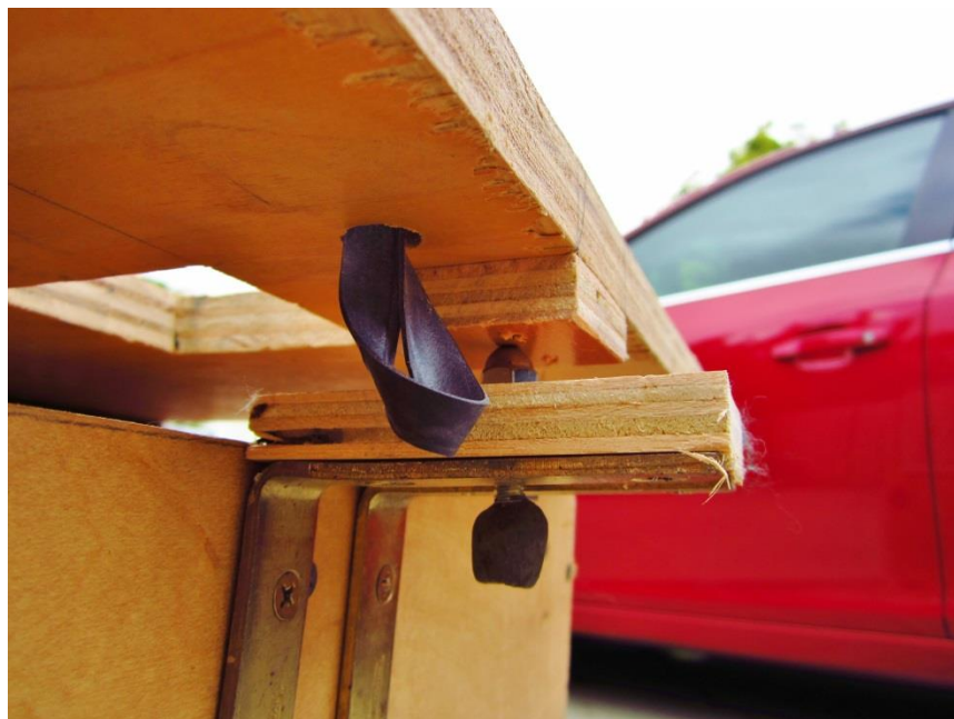
Figure 15: The declination control screw with a rubber pull-up band for the declination controller.
