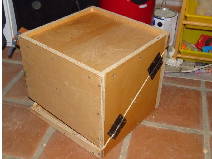
Figure 5: Barndoor box showing the hinges pointing at the celestial North Pole.
