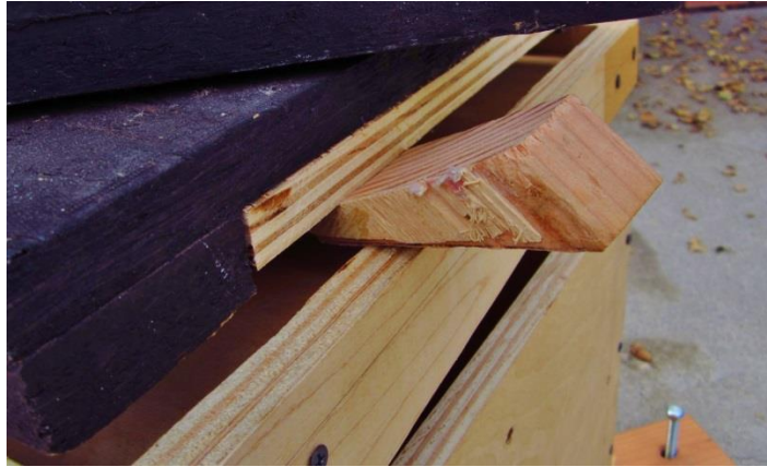
Figure 16: A wedge shaped piece of wood keeps the declination board from tipping while we are aiming at a target.
