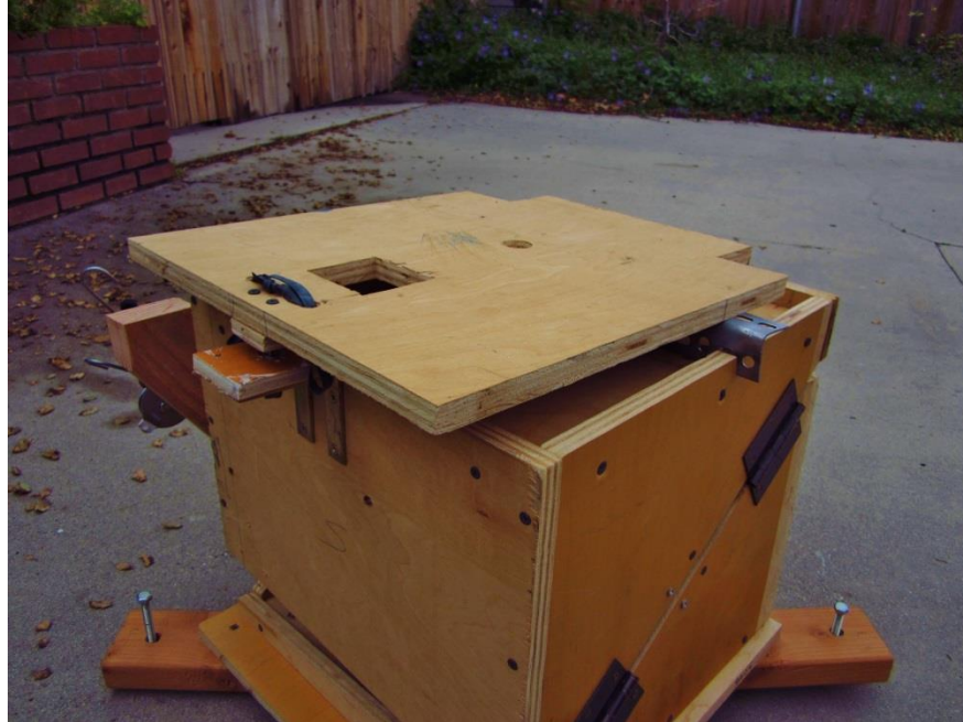
Figure 14: The declination board positioned at a place where it causes a narrow balance margin.
