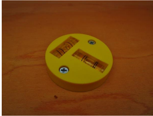
Figure 8: Bidirectional level attached to the base.
