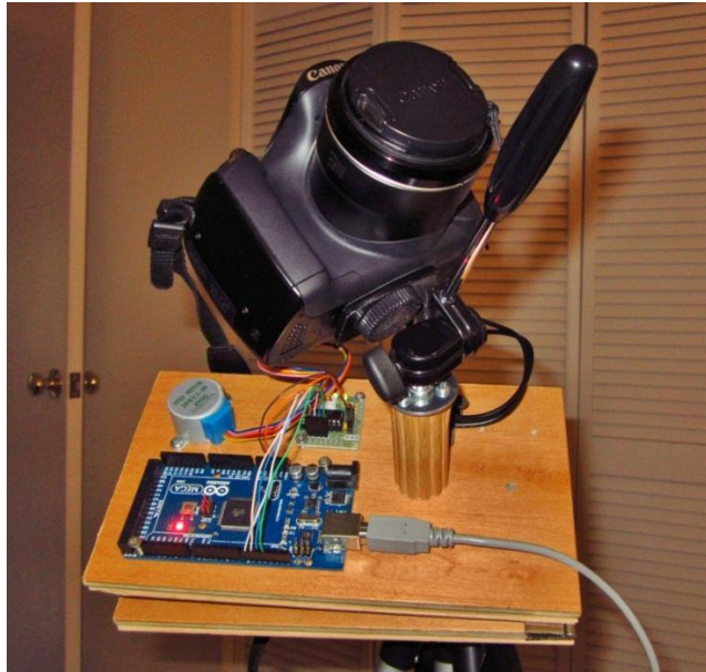
Figure 2: A traditional camera barndoor platform.
