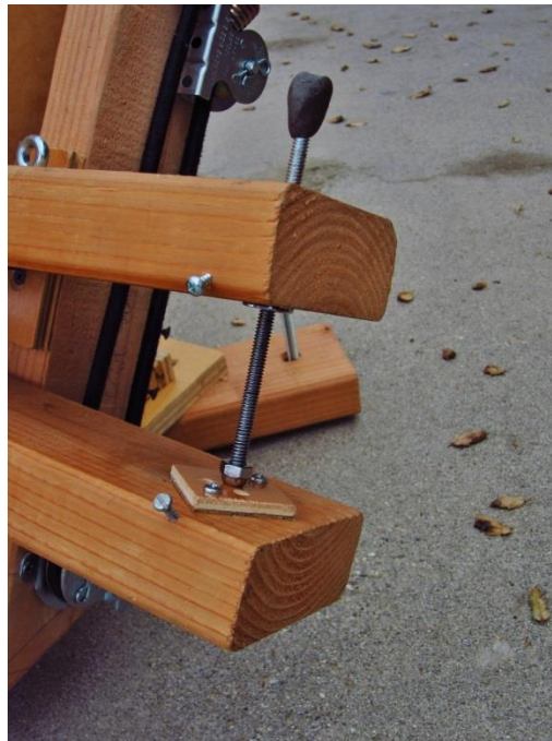
Figure 11: The screw rotates in a dimple in a small piece of floorboard. A glob of epoxy around the top has a hole in the shape of the stepper motor axis that was pressed into it.
